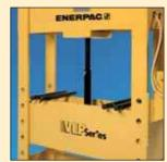
**Moveable pumptable** on presses with electric pumps allow for easy side loading of large workpieces.
