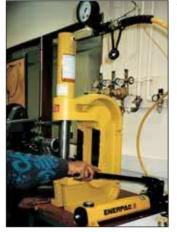
A-310 Abor Press used for compacting powder at 10 ton.
