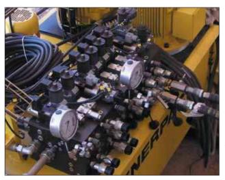
A typical multi-cylinder control set-up using solenoid directional control valves.
